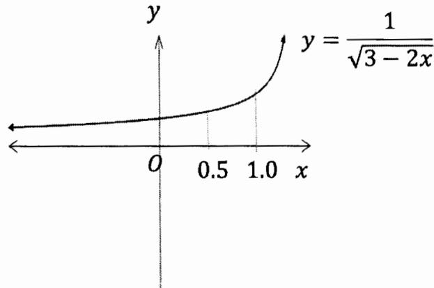
The diagram shows the graph of  $y = \frac{1}{\sqrt{3-2x}}$ . The region bounded by this graph,  $x = 0.5$ ,  $x = 1.0$  and the  $x$ -axis is rotated about the  $x$ -axis. Find the volume of the solid of revolution formed in exact form. 3
